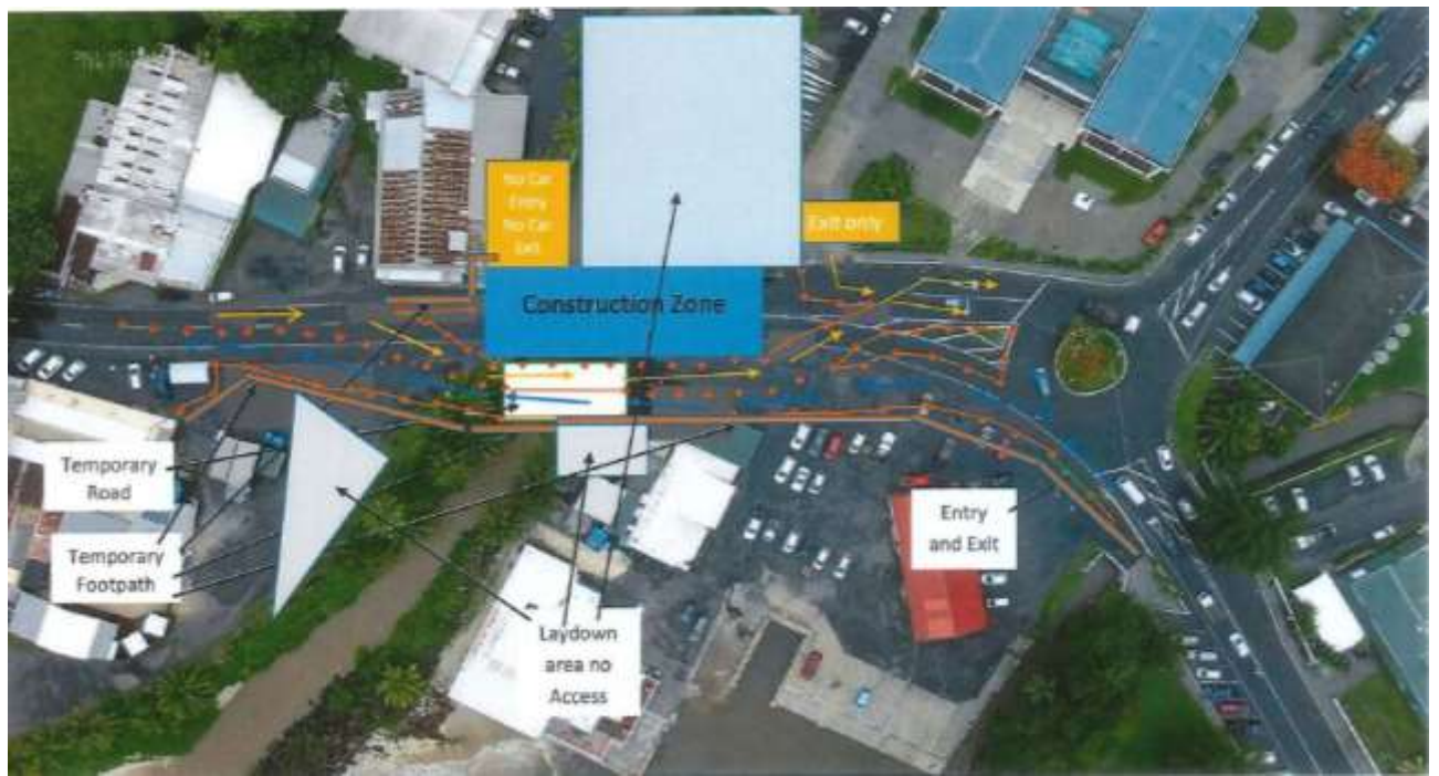
Figure 7: Contractors Traffic Management Plan
